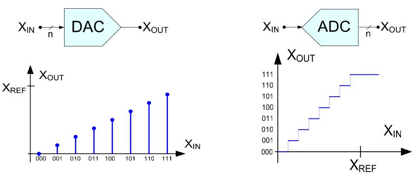
The LSB is the nominal value of the smallest change that occurs in the output of an ideal DAC or the nominal value of the smallest increment in the input that causes a change of a single binary digit in an ADC
